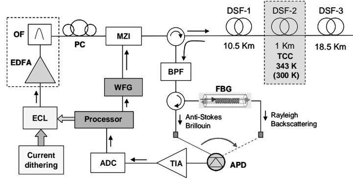
Fig. 3. Experimental set-up of the implemented sensor system.
